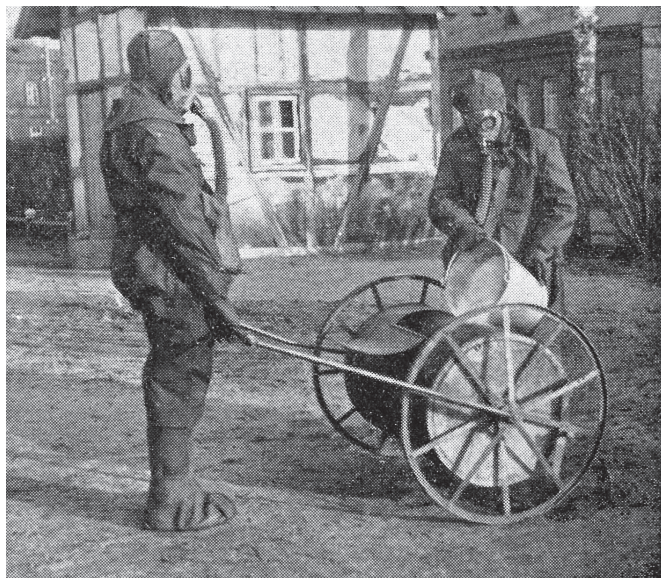
Figure 5. Degasers equipped with anti-mustard gas overalls filling up the chlorine lime roll. Source: KAREIVA, M[ečys]. Degazacija. Kaunas, 1937
