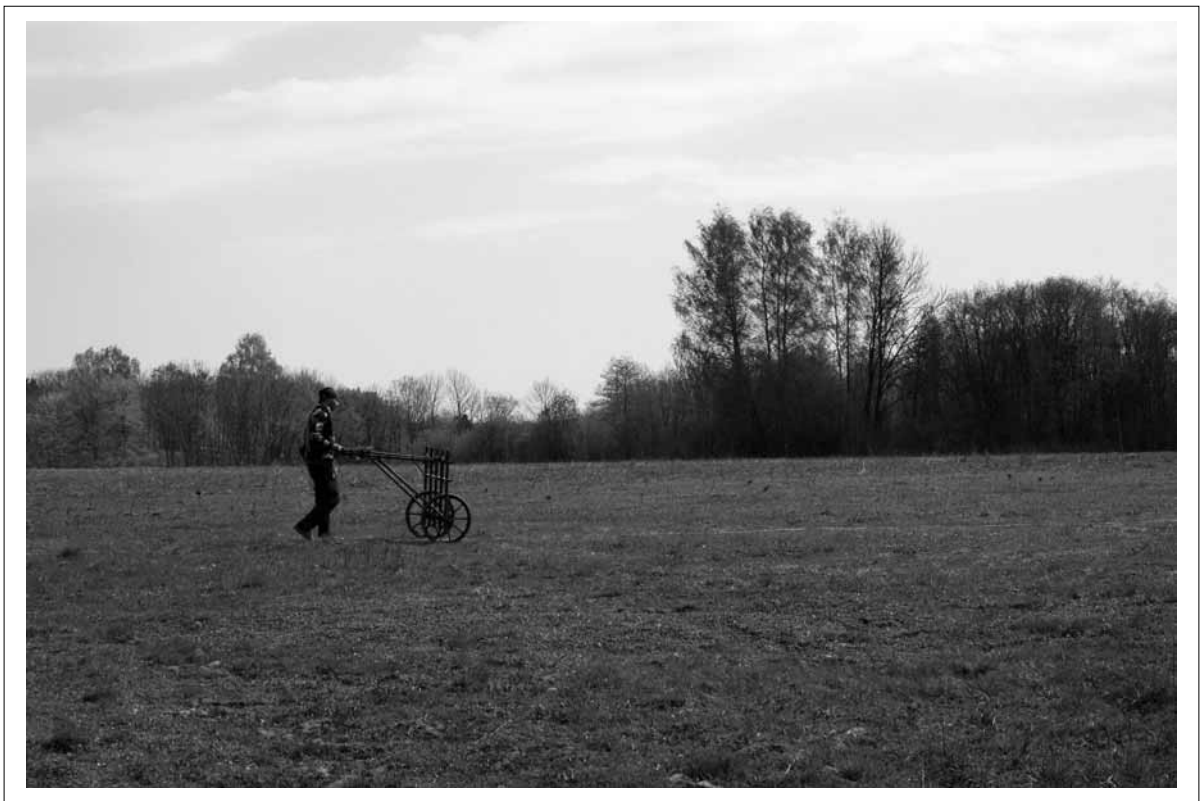
Fig. 2. Ēgliškiai-Anduliai. Geomagnetic survey with a five-channel magnetometer.
