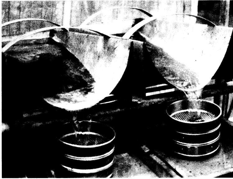
Fig. 4. A closer look at the flotation system. Photo David N. Simpson
