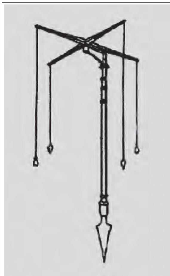
Fig. 3. (left) Funerary stele of a gromatic discovered in excavations at Pompeii, showing a schematic representation of his groma . (right) Idealized reconstruction of the instrument from different elements unearthed during excavations at the same site. (Adapted from Adam 2002).
