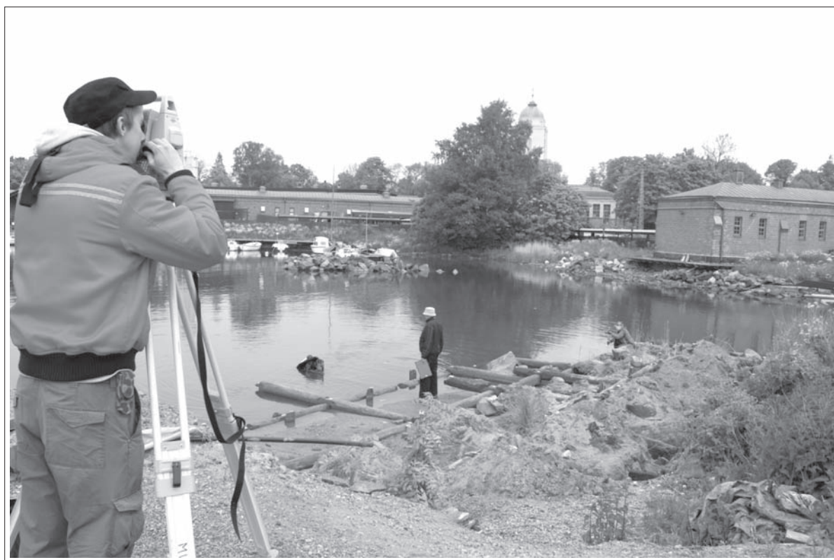
Fig. 5. Archaeological documentation on the smaller log-barrier embankment was carried out with the help of Total Station (photograph by M. Leino).
